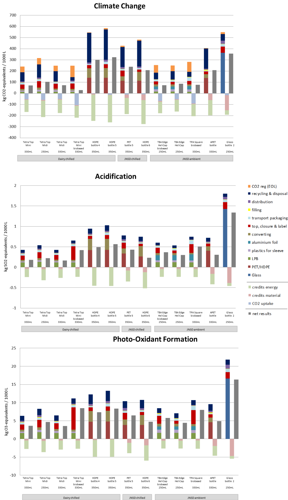
Figure 46: Indicator results for sensitivity analysis on system allocation of segment Grab & Go, Sweden, allocation factor 100% (Part 1)
