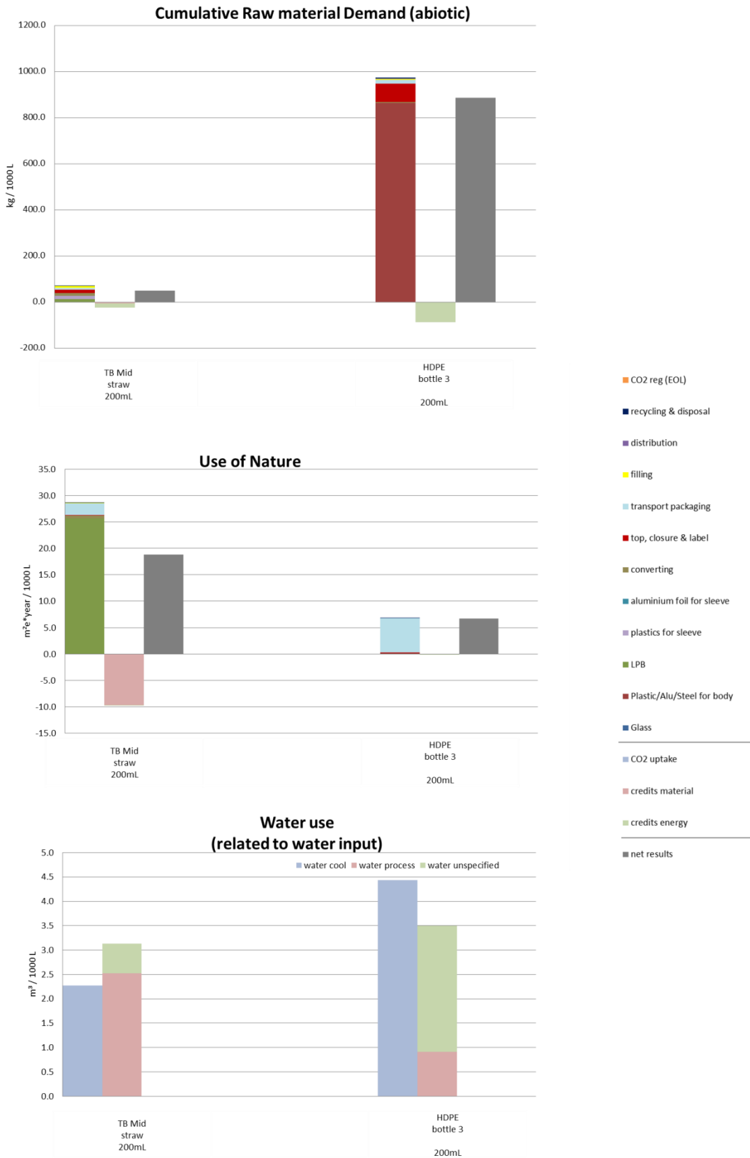
Figure 95: Indicator results for scenario variants regarding plant-based plastics in HDPE bottles of segment DAIRY PORTION PACK (chilled), Europe , allocation factor 50% (Part 4)
