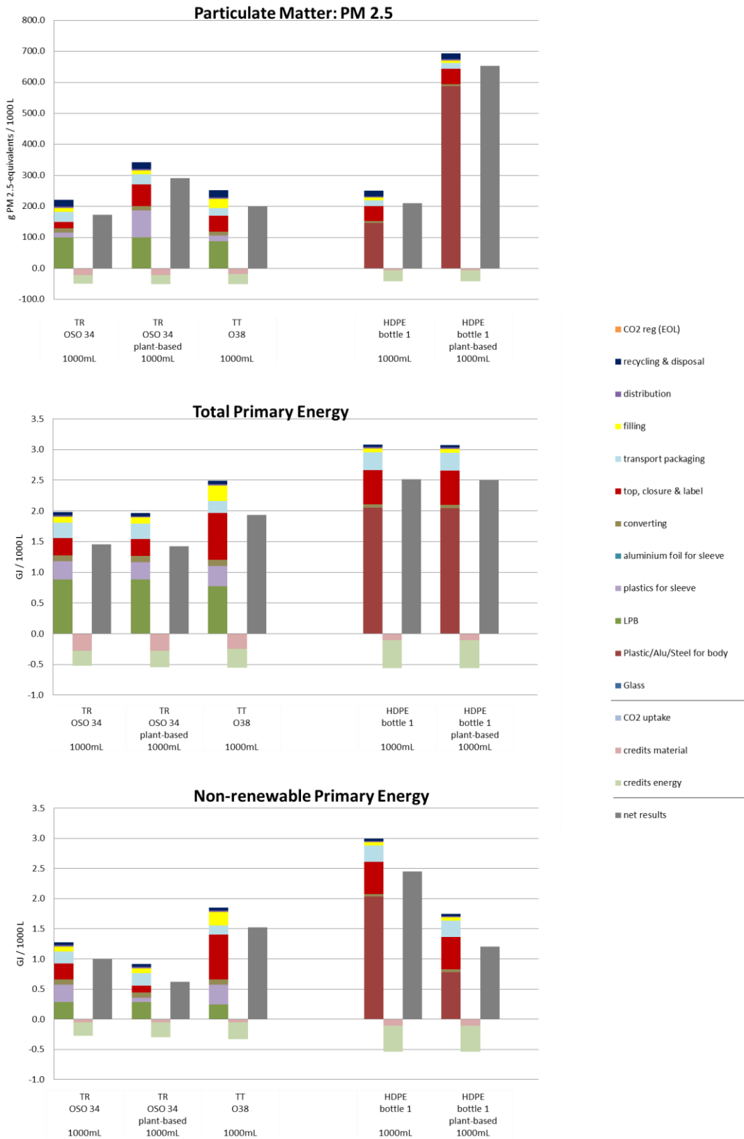
Figure 78: Indicator results for scenario variants regarding plant-based plastics in HDPE bottles of segment DAIRY FAMILY PACK (chilled), Europe , allocation factor 50% (Part 3)
