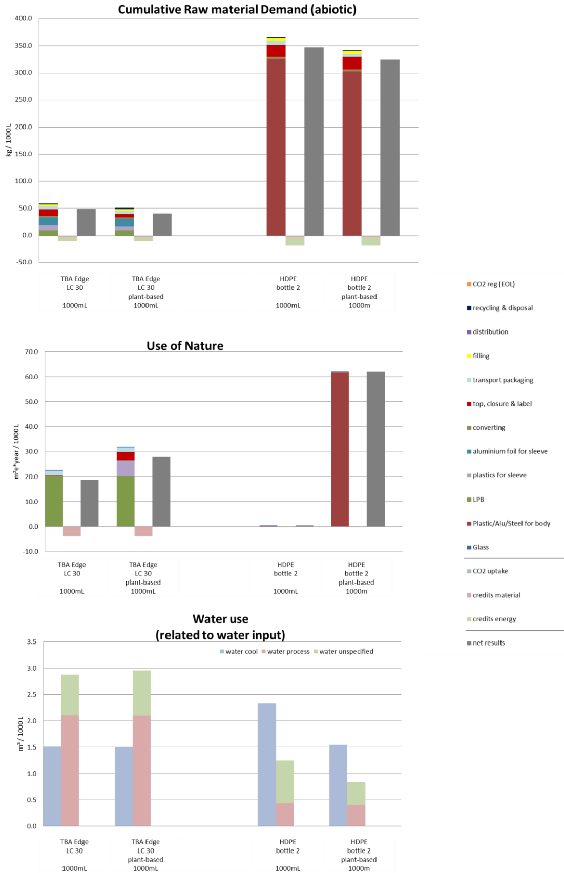
Figure 87: Indicator results for scenario variants regarding plant-based plastics in HDPE bottles of segment DAIRY FAMILY PACK (ambient), Europe , allocation factor 50% (Part 4)
