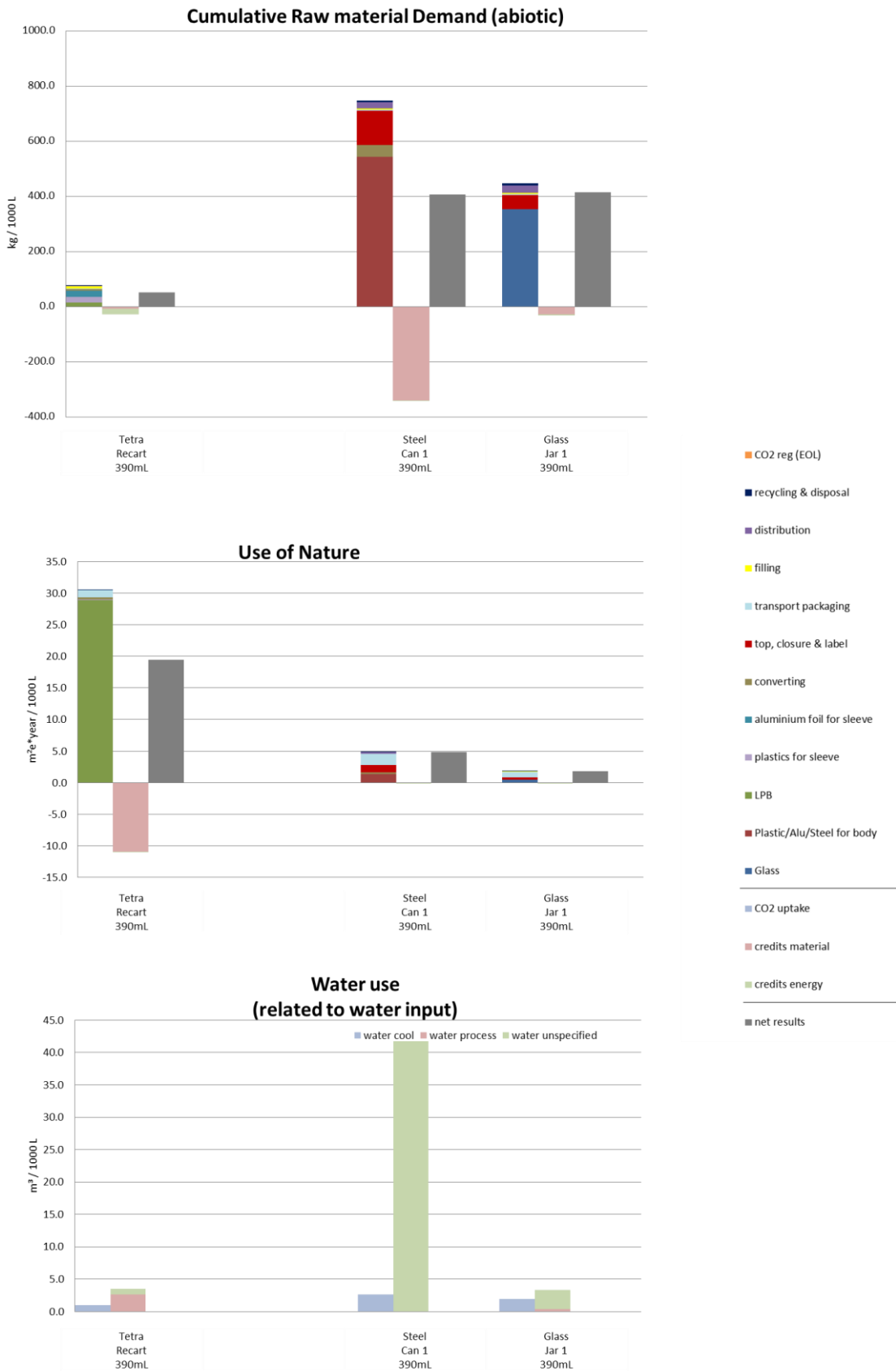
Figure 75: Indicator results for sensitivity analysis on system allocation of segment LIQUID FOOD PORTION PACK AMBIENT, allocation factor 100% (Part 4)
