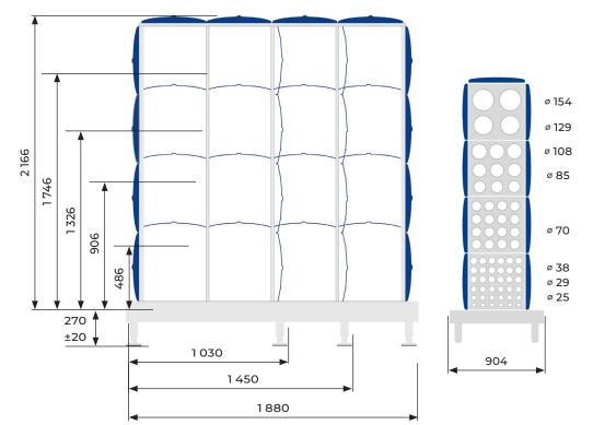
Tube modules with different shell diameters can be mounted on the same frame.
