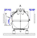
\*Keep the height of the platform to the manhole 1 000 mm the same for all manholes of the device. Example layout of the Tetra Pak® Grainy Cheese Vat E4 with maintenance area.
